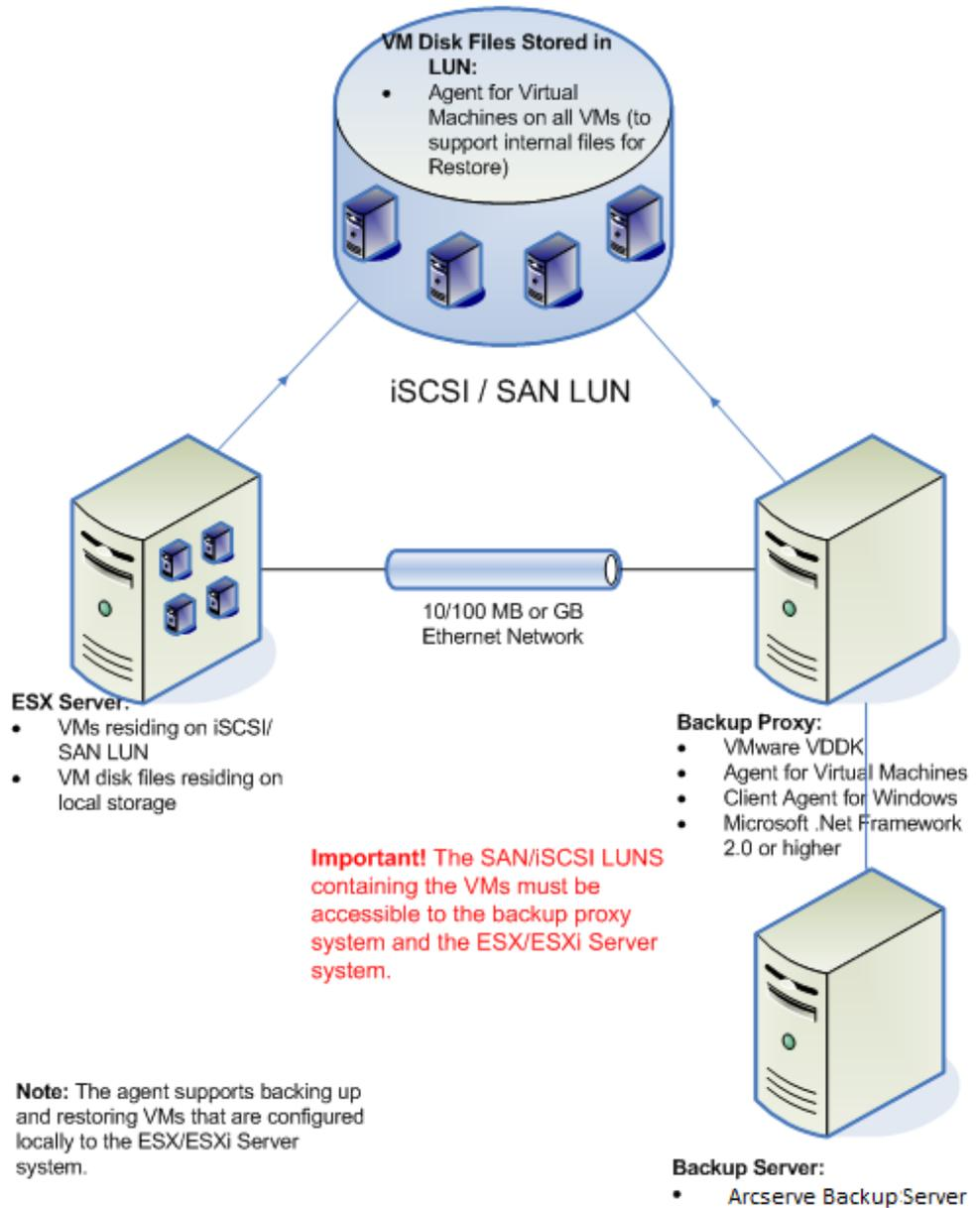
1. The Arcserve Backup primary or member server communicates with the Agent for Virtual Machines that is running on the backup proxy system while the backup job is running. The agent then takes a snapshot of the VM and mounts or exports the snapshot to the backup proxy system, by default, into the Client Agent for Windows installation directory.
