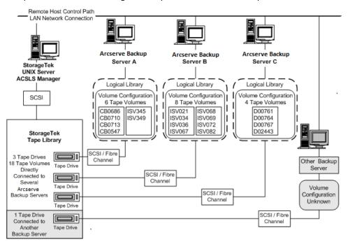
The example shows that the StorageTek ACSLS tape library has four tape drives directly attached to several backup servers on the network. The unique tape volume assignments for each Arcserve Backup server are:
