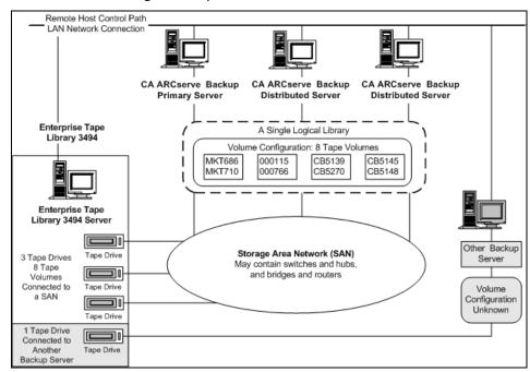
The example shows that the Enterprise Tape Library 3494 has three tape drives directly attached to a SAN. The tape volume assignments are the same for each Arcserve Backup server in the SAN. Another backup server on the network that is not running Arcserve Backup may have a different configuration.
