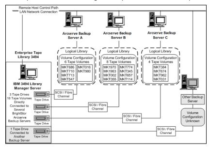
The example shows that the Enterprise Tape Library 3494 has four tape drives directly attached to several backup servers on the network. The unique tape volume assignments for each Arcserve Backup server are:
