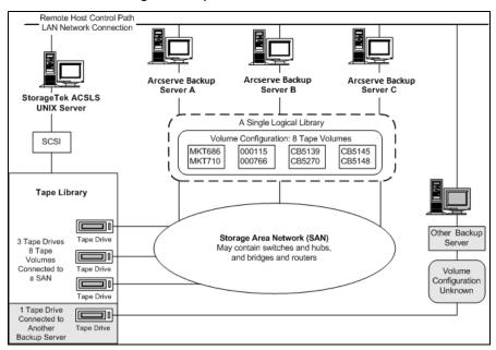
The illustration shows that the StorageTek ACSLS tape library has three tape drives directly attached to a SAN. The tape volume assignments are the same for each Arcserve Backup server in the SAN. Another backup server on the network that is not running Arcserve Backup may have a different configuration.
