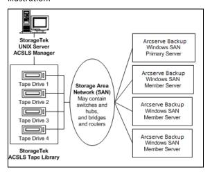
**Note:** In configurations where more than one tape drive is connected to a Arcserve Backup server, both tape drives must use media of the same type.
