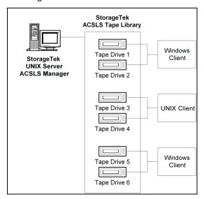
**Note:** In configurations where more than one tape drive is connected to a Arcserve Backup server, both tape drives must use media of the same type.
