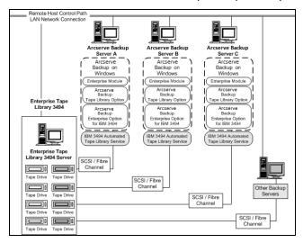
If multiple backup servers are sharing the same Enterprise Tape Library 3494, you must ensure that each tape volume is assigned to only one backup server. The tape volumes assigned to each backup server should be mutually exclusive, which means they cannot be used or accessed by other backup servers attached to the network.
