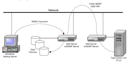
The following diagram shows an example of a three-way restore:
