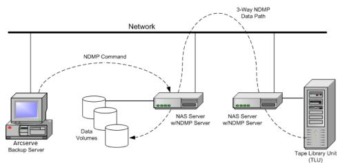
The following diagram shows an example of a three-way restore:
