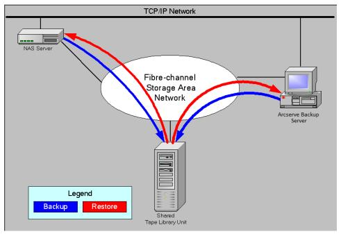
The following diagram shows an example of two or more NAS servers connected to the SAN that share a tape drive or TLU, and the Arcserve Backup server not connected to the SAN.
