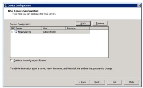
Steps 6 and 7 are optional steps for NAS servers supporting NDMP Versions 3 and 4. NAS servers which are enabled for NDMP Version 3 or Version 4 allow the client to detect backup devices that are configured on the NAS server. The NDMP NAS Option detects and displays all the detected devices. The format and usage rules governing the logical device names differ from one vendor to another. After you complete this step, DDS will be enabled for use.
