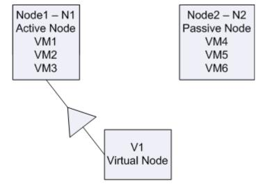
In an ideal scenario, virtual cluster node V1 directs network traffic to the active node (N1). When failover occurs, virtual cluster node V1 directs the network traffic to the passive node (N2), and all of the VMs in the active node (N1) move to the passive node (N2).
