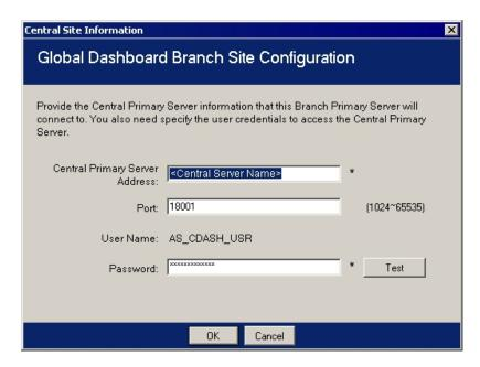
This dialog displays connection information to the central site. For a branch site to properly communicate to the central site, these parameters must be the same as specified for the central site configuration.
