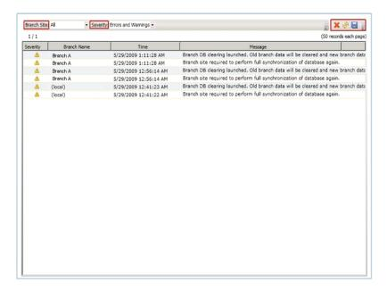
This listing can display log messages for all registered branch sites or can be filtered for just a specific branch site. This listing can also be filtered to display only messages for a specific severity level (All, Messages, Warnings, Errors, and Errors and Warnings).
