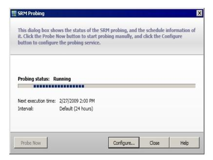
To configure the SRM Prober settings, click the Configure button. The Configure SRM dialog opens.
