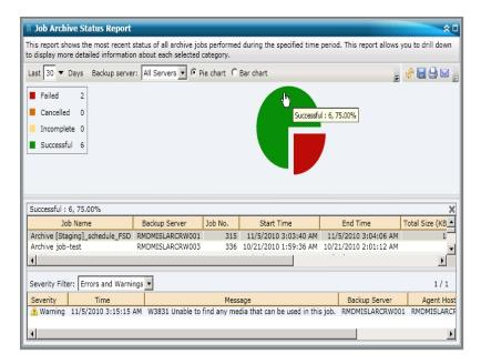
You can drill down further in this report by clicking on the name of an individual job to display a more detailed listing of all log messages associated with that job. You can also filter the list by specifying the severity of the messages displayed (Errors and Warnings, Errors, Warnings, Information, or All).
