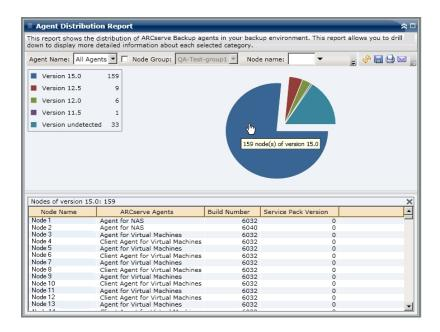
The Agent Distribution Report will only display the Service Pack (SP) version of nodes that have Arcserve Backup agents at r16.5 or later release. For the earlier releases, the SP information can be identified from the "Build" column in the report by using the following table to convert the build number to the corresponding SP number.
