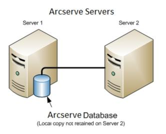
In the following diagram, multiple Arcserve Backup servers are sharing a centralized database. A copy of the Arcserve Backup database is retained on one of the servers sharing the database.
