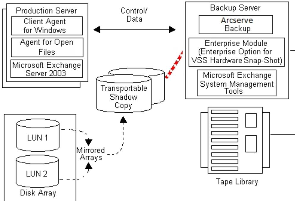
**Note:** The dashed line now represents the logical attachment between the Arcserve Backup server and the cloned data on the transportable shadow copy volume.
