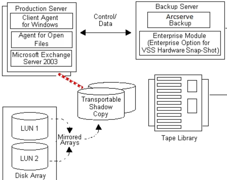
**Note:** The dashed line represents the logical connection between a Microsoft Exchange 2003 Server and the cloned data on the transportable shadow copy volume.
