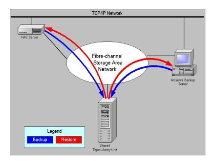
The following diagram shows an example of two or more NAS servers connected to the SAN that share a tape drive or TLU, and the Arcserve Backup server not con-
