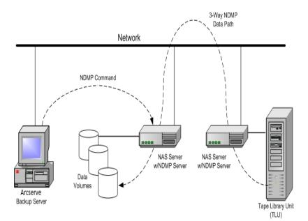
The following diagram shows an example of a three-way restore:
