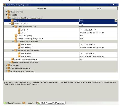
This is the IP address that the Master will switch over to. If you are moving more than one IP address you can add multiple production IP addresses by selecting Click here to add new IP/Mask.
