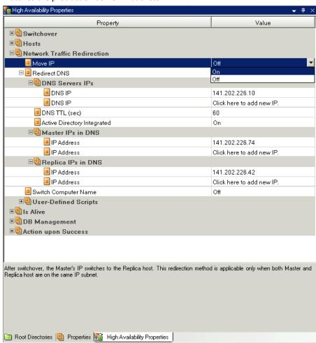
This is the IP address that the Master will switch over to. If you are moving more than one IP address you can add multiple production IP addresses by selecting Click here to add new IP/Mask.
