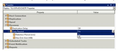
If this option is set to Off, the system will not register data rewind points. For more information about Data Rewind parameters (Retention Period, Max Disk Size), see the *Arcserve RHA* Administration Guide.
