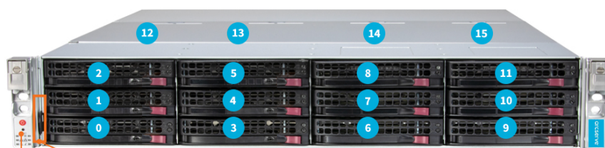
Control Panel IPMI password and Arcserve Appliance model number
