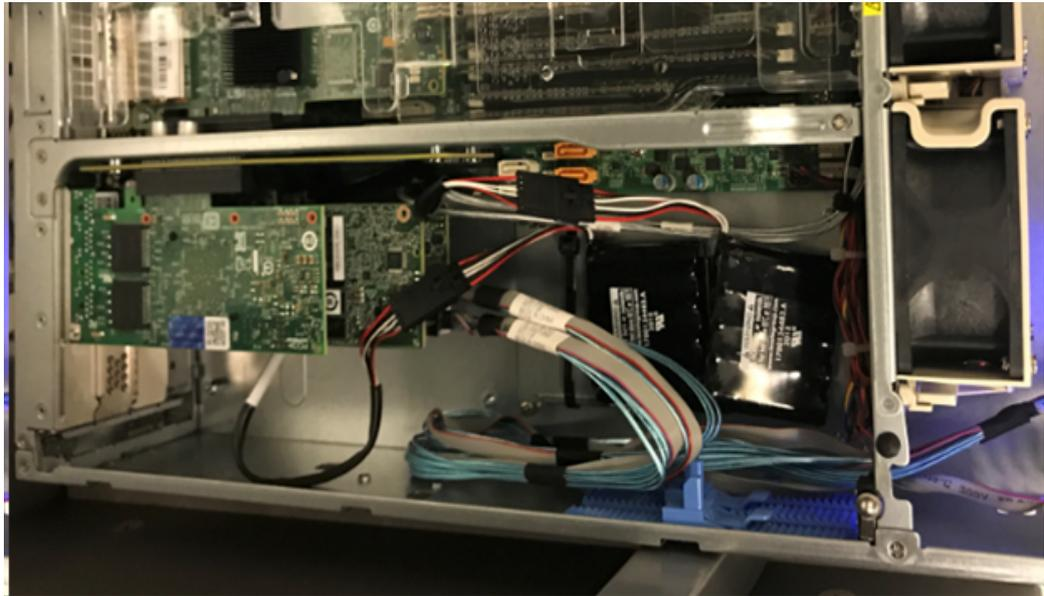
7. Secure the *MegaRAID Controller 9380-8e* bracket to the chassis of the system.
