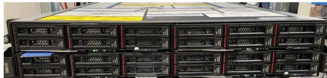
There are four nodes in a 2U chassis, each with six 2.5 inch form factor drive bays. Each node has a power button located below the node's center column drive bays. Full control of all nodes is available via a web browser using XClarity administrator.
