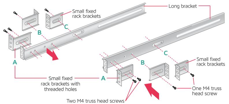
**NOTE:** Once the assembled rails are attached to the rack, securely tighten the single screws on steps B and C.
