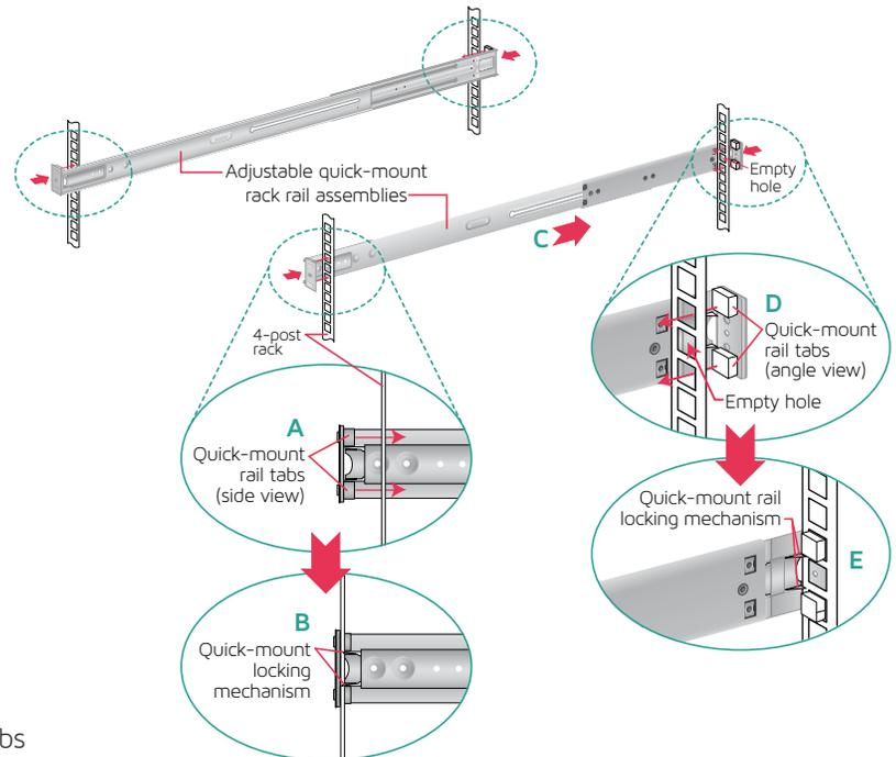
\* **NOTE:** Make sure the quick-mount rail assemblies are aligned in the rack not only in the front and back, but are level in height on the left and right sides for proper alignment for appliance installation.
