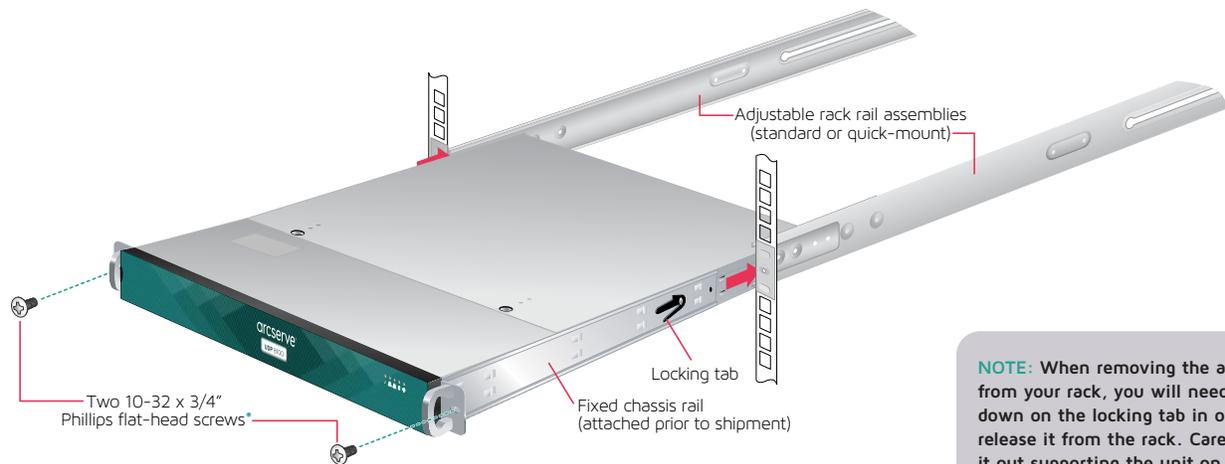
**NOTE:** When removing the appliance from your rack, you will need to press down on the locking tab in order to release it from the rack. Carefully slide it out supporting the unit on both sides at all times.
