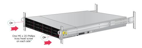
\* NOTE: Refer to your rack's mountiing hardware for the proper size and type of screws to secure the appliance in the rack if different from the screws supplied in this ship kit.
