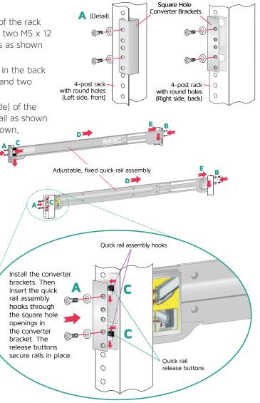
NOTE: The installation procedures for 6B, 4-Post Rack, below are for use with the rails and hardware provided in your ship kit. If different style rails are being used, or if your rack requires different hardware,
