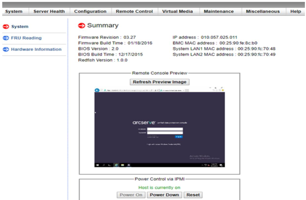
The screenshot shows the IPMI web interface with a navigation bar at the top containing: System, Server Health, Configuration, Remote Control, Virtual Media, Maintenance, Miscellaneous, and Help. On the left, there is a sidebar with links for System, FRU Reading, and Hardware Information. The main content area is titled 'Summary' and displays the following information:
