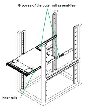
2. Slide the chassis rails into the rack rails until the chassis is completely in the rack.
