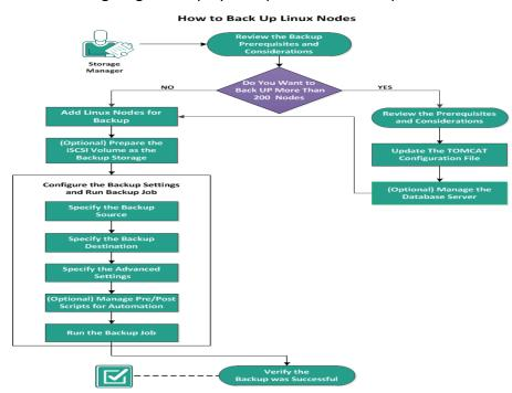
The following diagram displays the process to back up Linux nodes:
