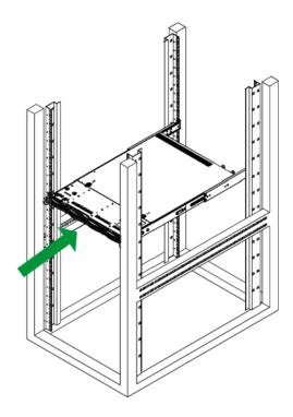
**Note:** Figure is for illustrative purposes only. Always install servers to the bottom of a rack first.
